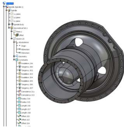
Figure 3. 3D CATIA model with corresponding product tree
